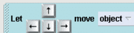
FIGURE 6: The built-in Alice event to let the arrow keys move an object
